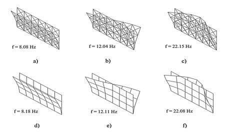
Figure 8 - Tuning of the out-of-plane stiffness in the enriched-ERC modeling. The enriched-ERC model (a, b, c) have same dimensions, mass and mesh-size of the shell model (d, e, f). The moments of inertia (Jxx and Jyy) and the torsion inertia moment (JT) of the added vertical beam-layer are tuned in order to reproduce (a, b, c) the first three modal frequencies and shapes of the "reference" shell model (d, e, f). Reproduced from [14].
