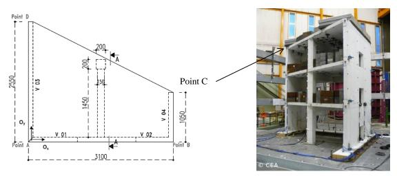
Figure 7- SMART mock-up[13]. Drawing related to a storey of the structure (left). General view of the experiment (right).
