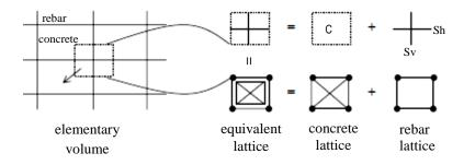
Figure 3- Equivalent Reinforced Concrete modeling [8].
