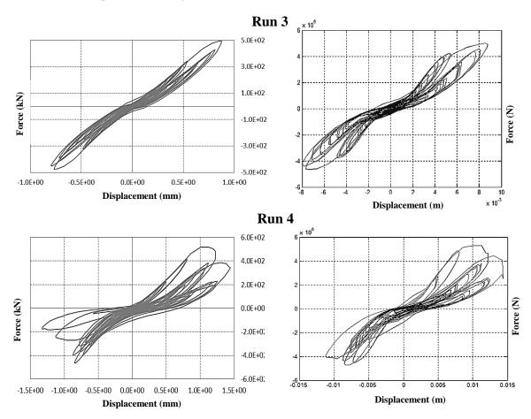
Figure 6- Overall force-displacement behavior of the SAFE wall in cyclic loading (Run 3 and 4). On the left, experimental response, on the right, numerical response.
