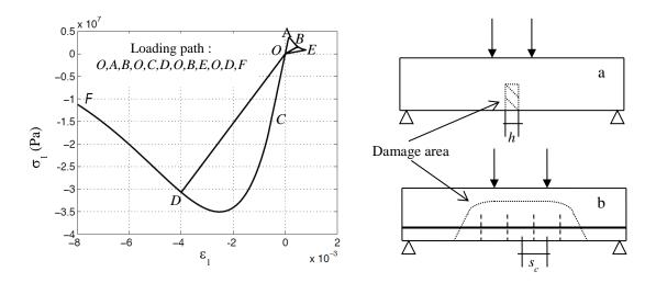
Figure 1(on the left) - Tension-compression loading path exhibiting the unilateral effect. Figure 2 (on the right) - Localization processes in a multi-fiber beam description; a) plain concrete: damage is localized in a band of elements (size h); and b) reinforced concrete: damage is distributed along the cracking zone ( $s_c$  is the crack spacing)
