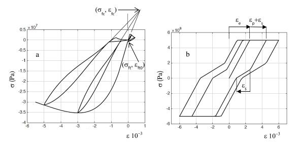
*Figure 4 – Enhanced constitutive 1D models: a) concrete curve including hysteretic loops and permanent strain; b) rebarconcrete bond curve obtained by introducing a sliding stage into the global steel fiber behavior.*
