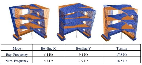
Figure 9- Vibration modes of the mock-up on the shaking table (for better clarity, the shaking table and the additional masses are not visualized): a) bending X-direction; b) bending Y-direction; c) torsion. Reproduced from [14].
