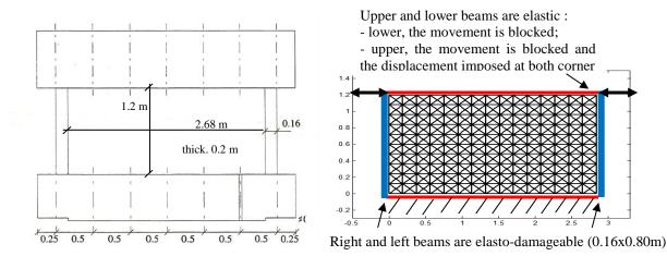
Figure 5- Scheme of the wall to be modeled and the selected discretization.
