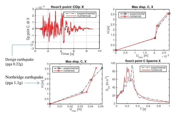
Figure 10- Experimental vs. numerical comparison - RUN 9, design earthquake: a) displacement history at point C, third floor, X-direction; b) maximum displacement at each floor, point C, X-direction - RUN 19 (Northridge earthquake): c) maximum displacement at each floor, point C, X- direction, and d) acceleration spectrum at point C, third floor, X-direction.
